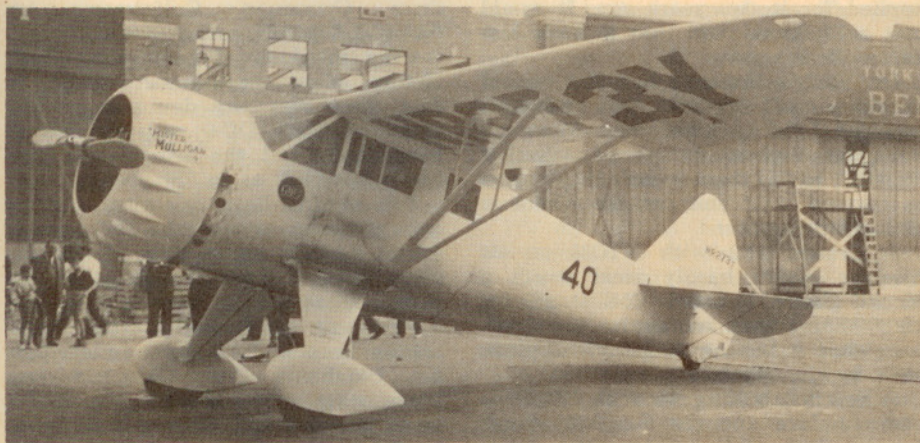
The Howard DGA-6 "Mr. Mulligan," sensation of the 1935 National Air Races. Built for racing but designed with commercial applications in mind, "Mulligan" bore a strong resemblance to a fattened-up version of the well-known Monocoupe.
