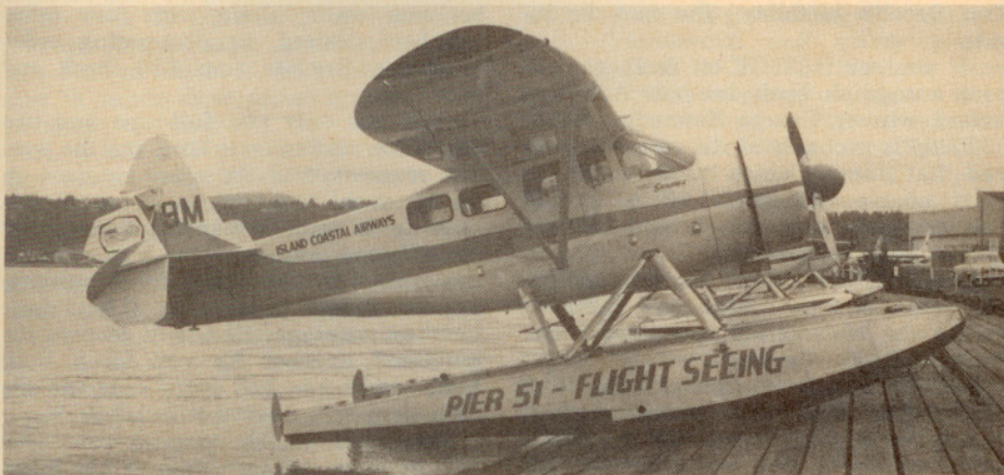
The civil DGAs were not intended to be seaplanes, but the Jobmaster Corp., Renton, Wash., worked out an approved Edo float installation in the early 1950s. Several "Jobmasters" are still operating in the Northwest.
